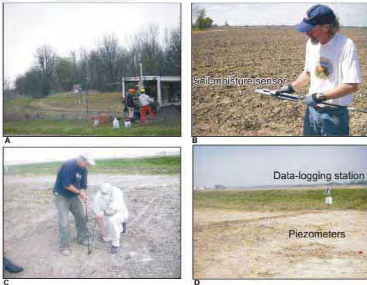
Figure 5. Installation of unsaturated-zone monitoring instruments at the Bogue Phalia River Basin, Mississippi study sites: (A) direct-push rig used to collect cores for installation of piezometers and soil-moisture sensors (looking west along piezometer transect at the southern study site); (B) sensor and insertion tool; (C) insertion of sensor; and (D) data-logging station for recording sensor data, and flush-mounted unsaturated-zone and water-table piezometers.
