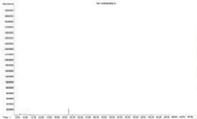
Figure 4. Chromatogram of NIST standard with ice plugging problem.
