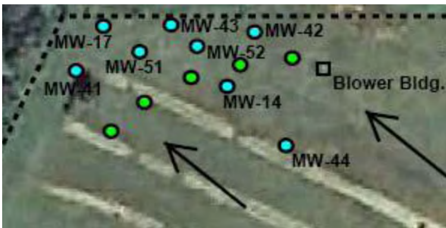
Figure 1. Aerial view of study site, indicating monitoring wells (MW- #), air sparging wells (unlabeled), and groundwater flow direction (arrows).
