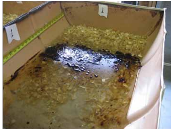
Figure 4. Test 1, (top left) shavings applied over sand, (top right) shavings sink when contacted by water and the oil floats over the top, (bottom left) as the water is removed simulating tidal movement, the oil is deposited on the shavings, (bottom right) the sand is protected as a sample is collected for analysis.
