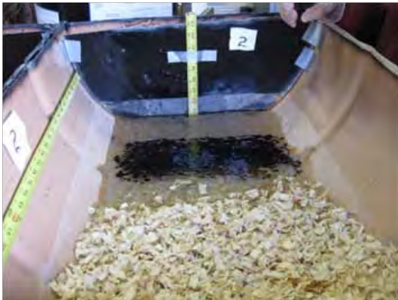
Figure 4. Test 1, (top left) shavings applied over sand, (top right) shavings sink when contacted by water and the oil floats over the top, (bottom left) as the water is removed simulating tidal movement, the oil is deposited on the shavings, (bottom right) the sand is protected as a sample is collected for analysis.
