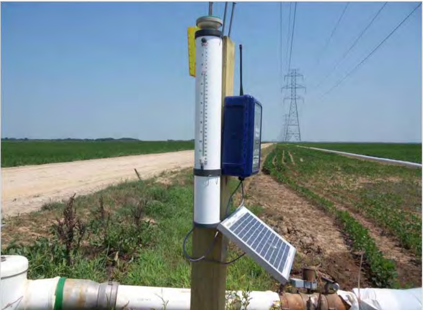
Figure 4. Evapotranspiration (ET) gauge equipped with data logger to estimate daily ET values and to schedule irrigation.
