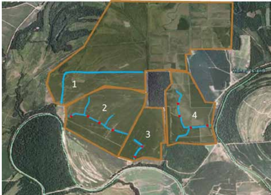
Figure 1. Aerial view of study site. Ditches are shown in blue, with the corresponding drainage areas outlined in red. Weirs are shown as red dots along the ditches. Tchula Lake is shown as a sinous white line at the southwest (bottom-left) and east (right).
