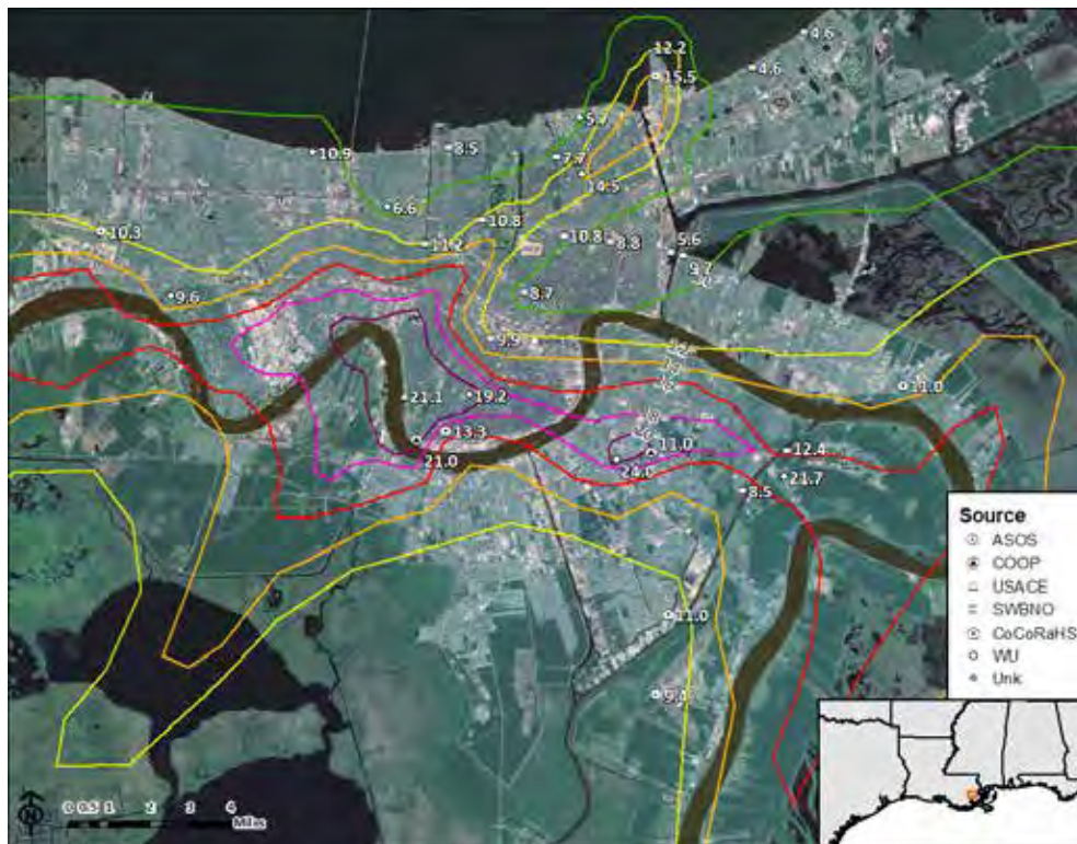
Figure 16. Storm total rainfall reported from all official and private gauges in the New Orleans area during Hurricane Isaac. Contours were produced from a Kriging interpolation of all official and private gauges. Note the particularly high values evident along the Mississippi River from roughly Gretna to Audubon Park.
