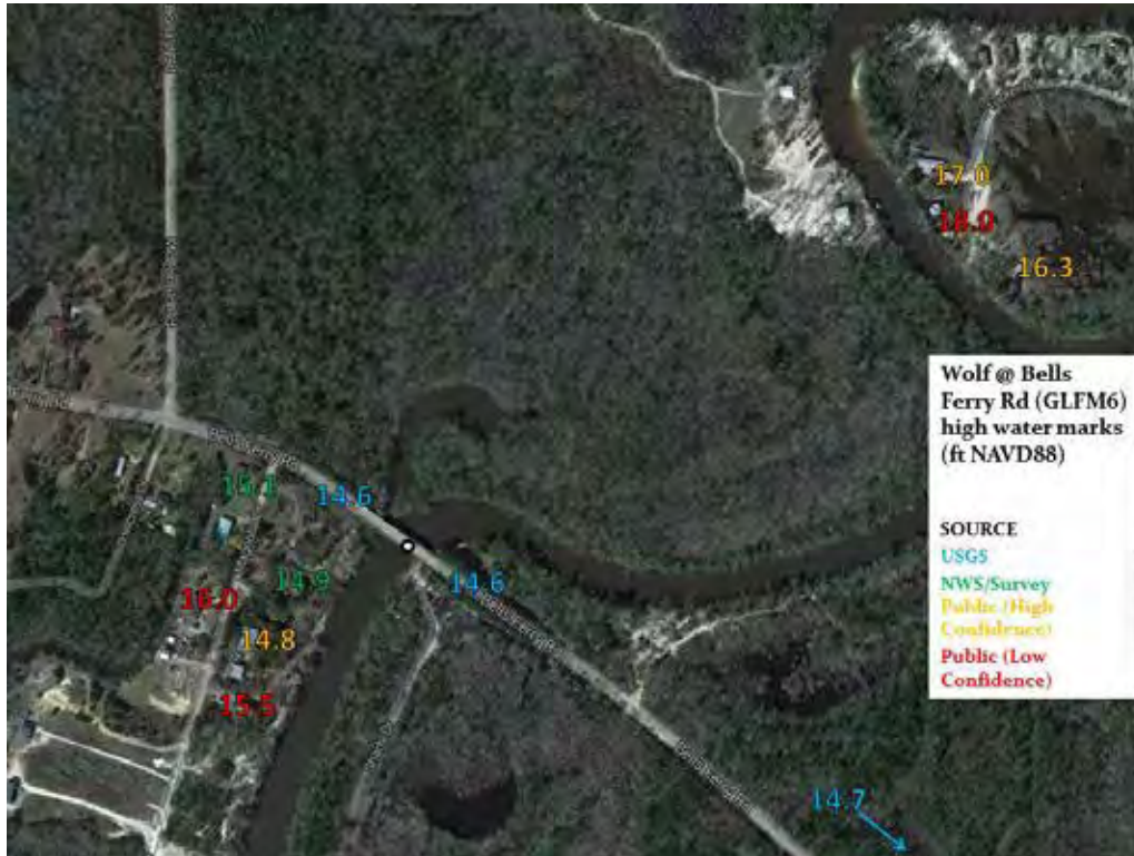
Figure 9. High water marks near the Wolf River at Bells Ferry Rd (GLFM6) gauge color-coded by confidence level. High water marks were adjusted to NAVD88 based upon the assumed staff gauge datum of -1.0 ft NAVD88.
