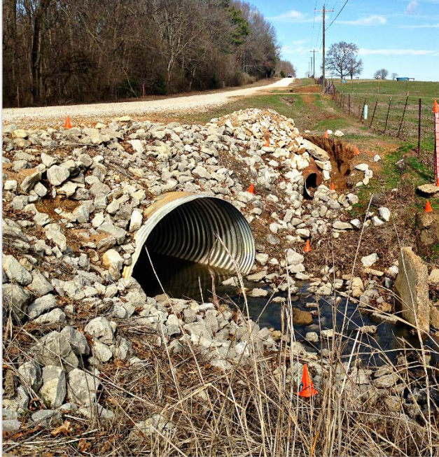
Figure 3. Soccer cones were placed at varying heights throughout the study area to serve as ground control points for vertical and horizontal accuracy of Structure from Motion digital surface models. The soccer cones were highly visible, inexpensive, and easy to deploy, but they were not durable enough for the environment.
