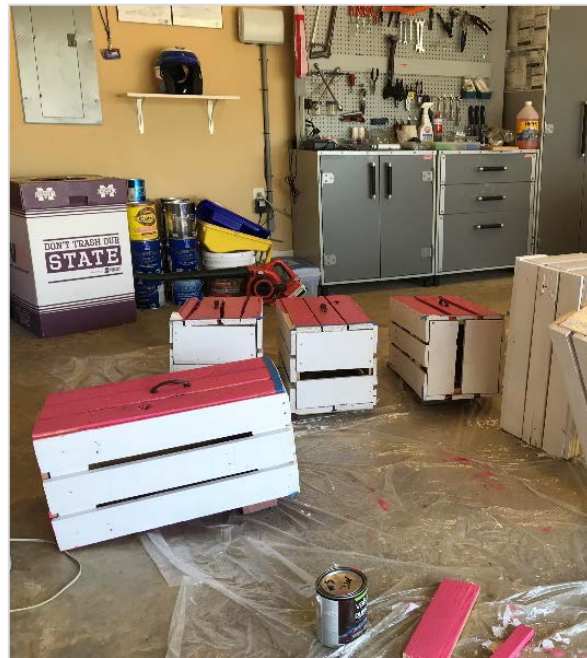
Figure 5. Calibration boxes were built from scrap materials and painted for high levels of visibility. While these large boxes were not suited for ground control points, they were useful in assessing the accuracy of volume estimates from the Structure from Motion digital surface models.
