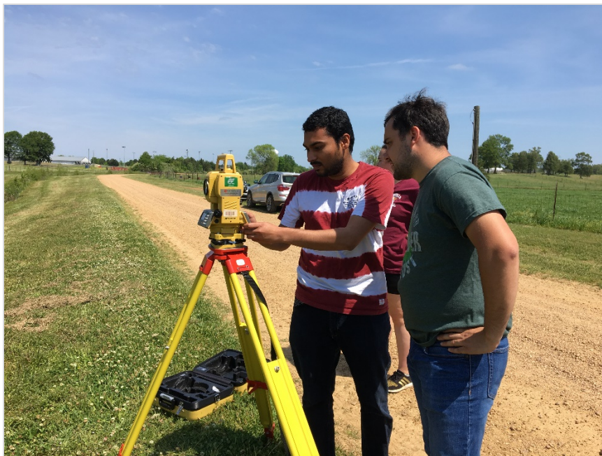
Figure 2. Students who participated in this project had previous classroom experience with use of survey equipment. Following a brief refresher course from an instructor in the Civil and Environmental Engineering Department, we utilized a total station and reflector survey poles to gather cross sectional elevations from our monitored tributary to Catalpa Creek.
