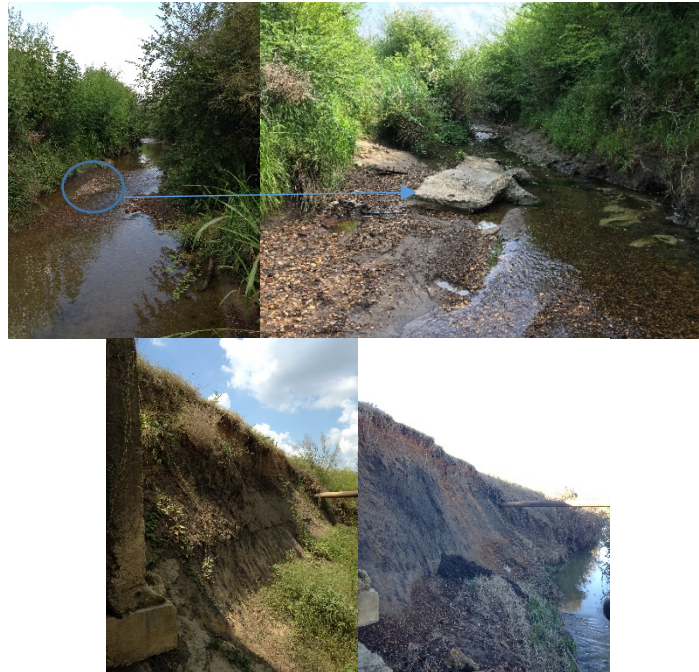
Figure 19. Upper picture evidences initial coarse material aggradation and posterior streambank toe and streambed degradation (erosion). As a reference, the rock in the middle part of the image was fully covered by sediment at the beginning of the study. Lower picture evidences streambank instabilities along the main stream of Catalpa Creek.
