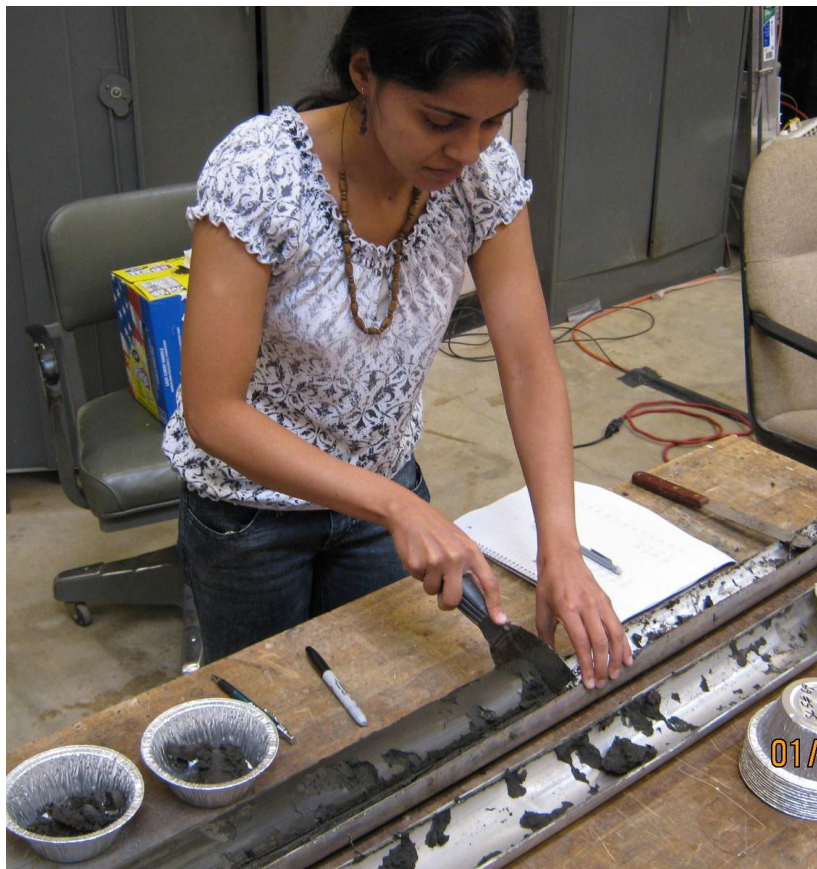
Figure 4. Sky Lake sediment core (SL5) being sliced into 1cm intervals at the National Sedimentation Laboratory.
