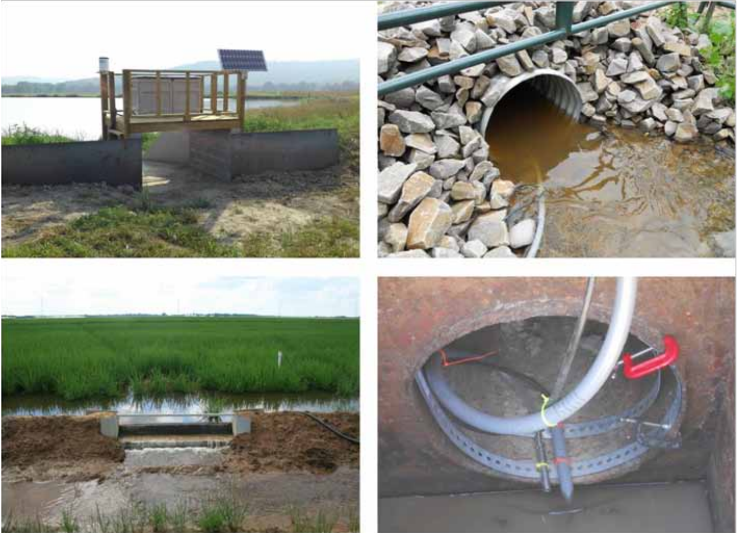
Figure 1. Various flow structures used in the Arkansas Discovery Farm program to quantify runoff volume: a) 3.5 foot h-flume to collect runoff from around poultry houses, b) culvert under cattle crossing to collect runoff from pasture (Manning's Equation), c) rectangular weir in rice field (also flood depth control and d) monitoring open channel pipe flow from soybean field; sampling strainer and pressure transducer are also shown for collecting water samples.
