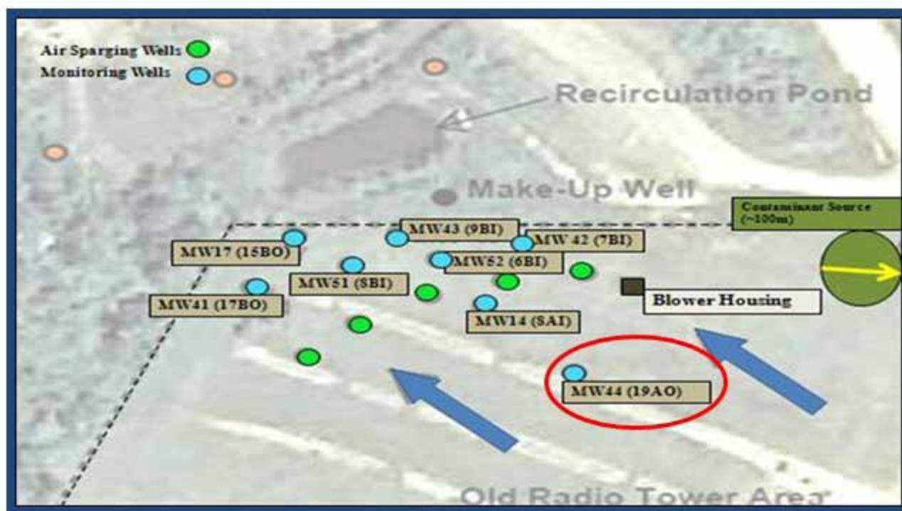
Figure 1. Aerial photograph of study site, including locations of biosparging wells and monitoring wells. Water sample for this study was collected from MW44 circled in red. Study site is located in central Mississippi and had initial PCP groundwater concentrations of ~3ppm(Stokes 2011)
